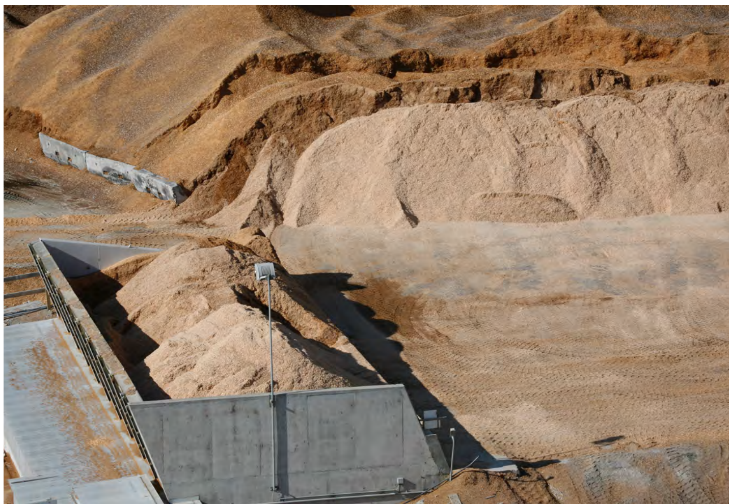
Wood waste (biomass) at Golden Bay Cement's Portland works is used as a partial replacement for coal as kiln fuel.
