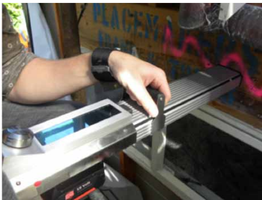
New generation microdrill checking doubled joist
