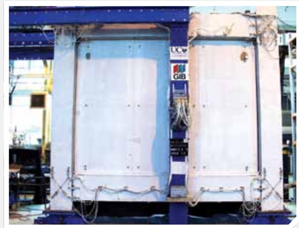
Figure 2: Non-structural partition being tested at Canterbury University
