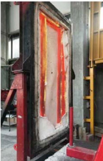
LEFT: Steel studs glow red-hot immediately following a pilot-scale furnace test. MIDDLE: A timber framed specimen at the end of a full-scale furnace test. RIGHT: Thermocouples collect important temperature data.
