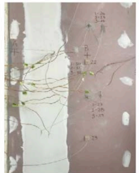
LEFT: Steel studs glow red-hot immediately following a pilot-scale furnace test. MIDDLE: A timber framed specimen at the end of a full-scale furnace test. RIGHT: Thermocouples collect important temperature data.
